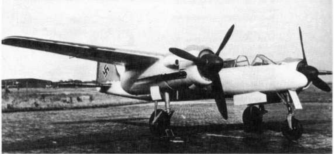
The Mosquito inspired a German imitation, the Focke Wulf Ta 154 Moskito, which, like the original, was constructed of wood.
