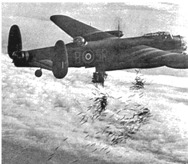
The Lancaster I NG128 dropping its load over Duisburg on Oct 14, 1944. The aircraft is carrying Airborne Cigar (ABC) radio jamming equipment, as shown by the two vertical aerials on the fuselage.
