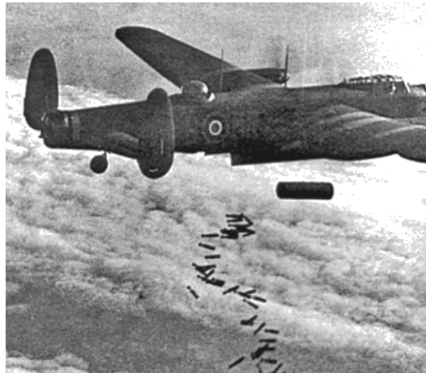
The Lancaster I NG128 dropping its load over Duisburg on Oct 14, 1944. The aircraft is carrying Airborne Cigar (ABC) radio jamming equipment, as shown by the two vertical aerials on the fuselage.
