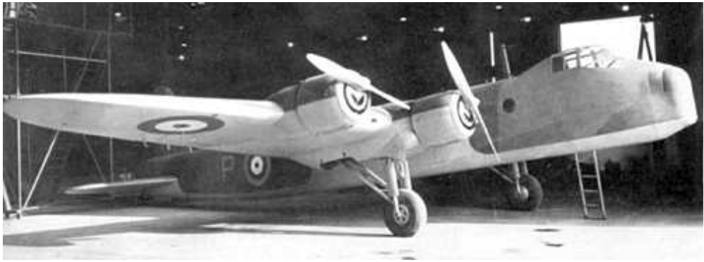
The Short S.31 half-scale replica used for aerodynamic tests of the Stirling design.
