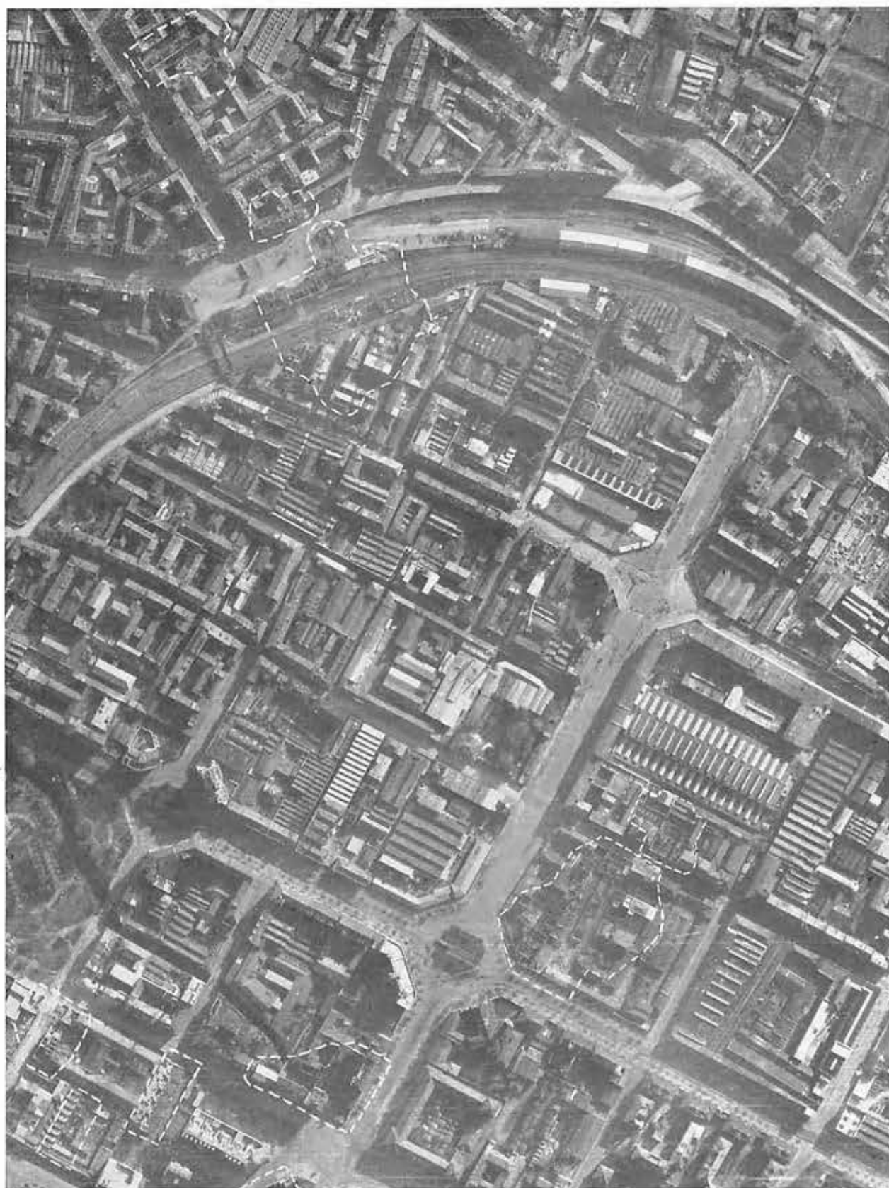
FIG. 11.—Industrial buildings suffered more heavily than residential and commercial buildings in the daylight attack. Photographs taken during the raid showed a concentration of incendiary sticks near the Electricity Works where a large fire occurred (see outlined area above, lower right). A 4,000-lb. H.E. bomb was shown to have fallen at the Genoa Railway Station, which was also damaged by fire (upper part of above photograph).
