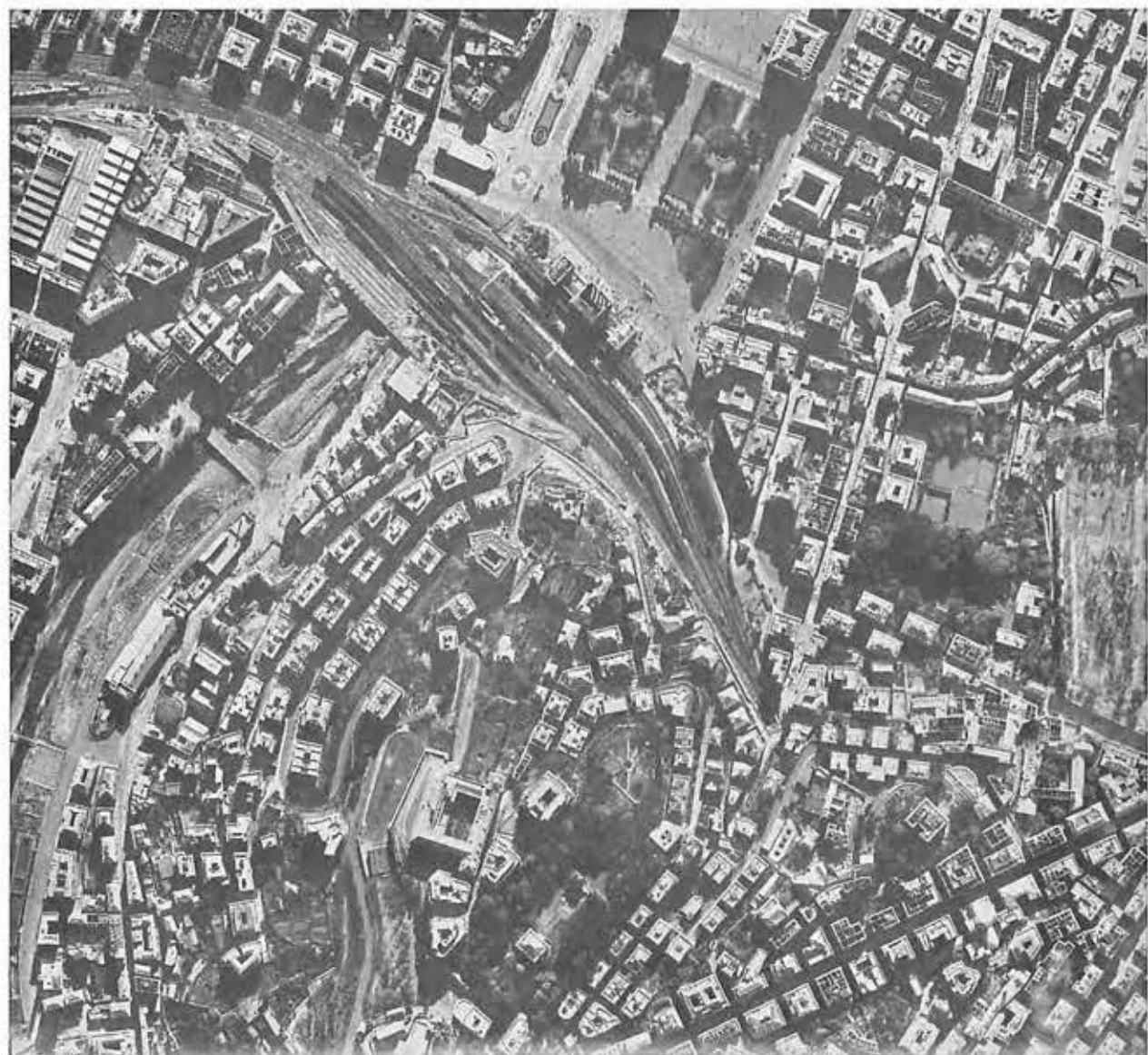
FIG. 5.—The neighbourhood of the Brignole Railway Station in the east part of the city shows many ruined buildings. At the station itself the main block was almost completely burnt out and platform buildings and tracks heavily damaged, part of a train destroyed and trucks on the sidings burnt out.
