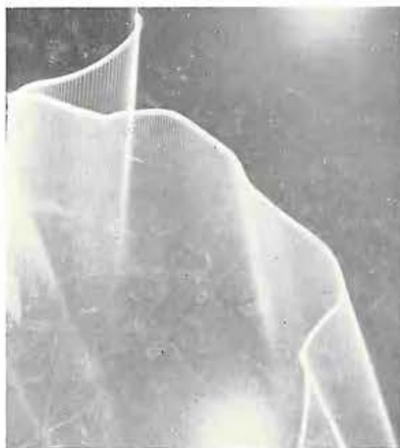
FIG. 41.—Searchlight over Düsseldorf. The curtain-like image is caused by the beam striking haze or mist, the "hem" is the track of the bowl. The beam has moved while the aircraft flew over. (R/83; 31.7/1.8.42.)
