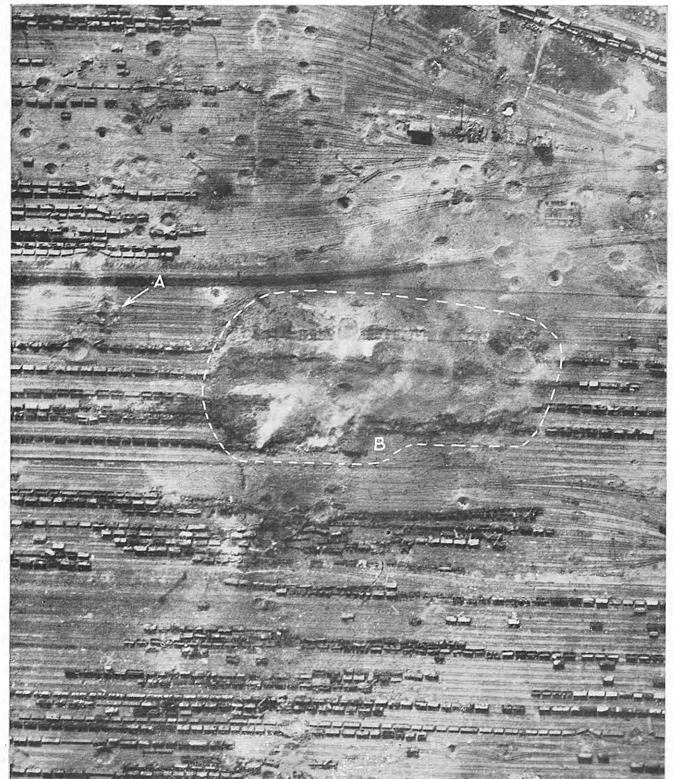
FIG. 12.—Reconnaissance showed that the great explosion in Vaires forwarding sidings resulted from the detonation of two munition trains. The area of complete devastation (B) measures about 250 yards by 150 yards.
