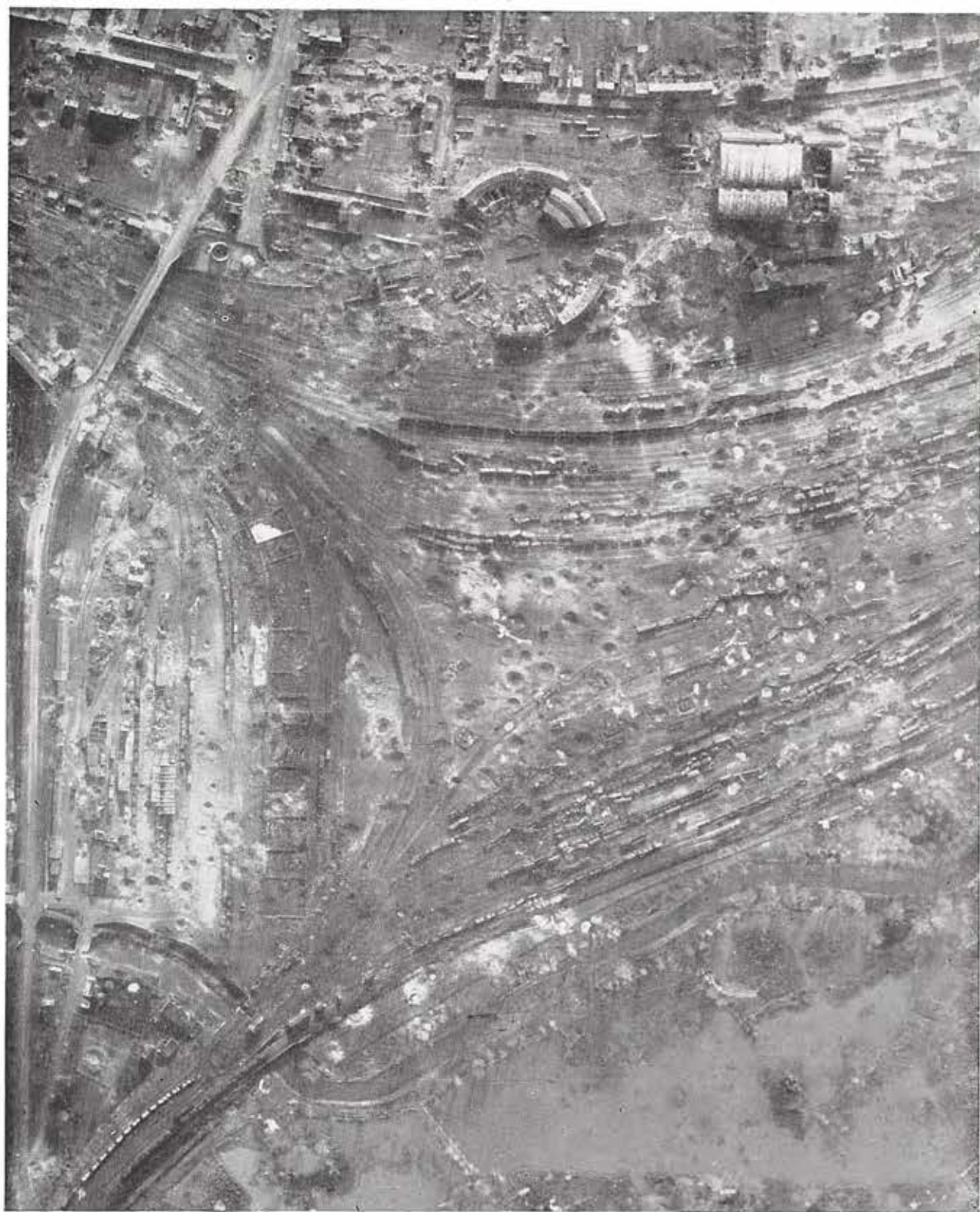
FIG. 9.—Enlarged view of area " B " on Fig. 10 ( opposite ). The turntable and engine sheds have been severely damaged, together with much of their contents. All tracks were cut in many places and few wagons escaped damage. The whole area of the railway yards was plastered with bomb-craters.
