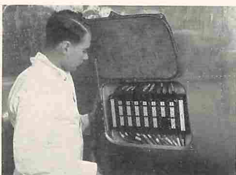
Main junction box, starboard side, with wiring diagram on door.
