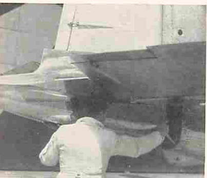
Removing tail-cone, held by four toggle fasteners.
