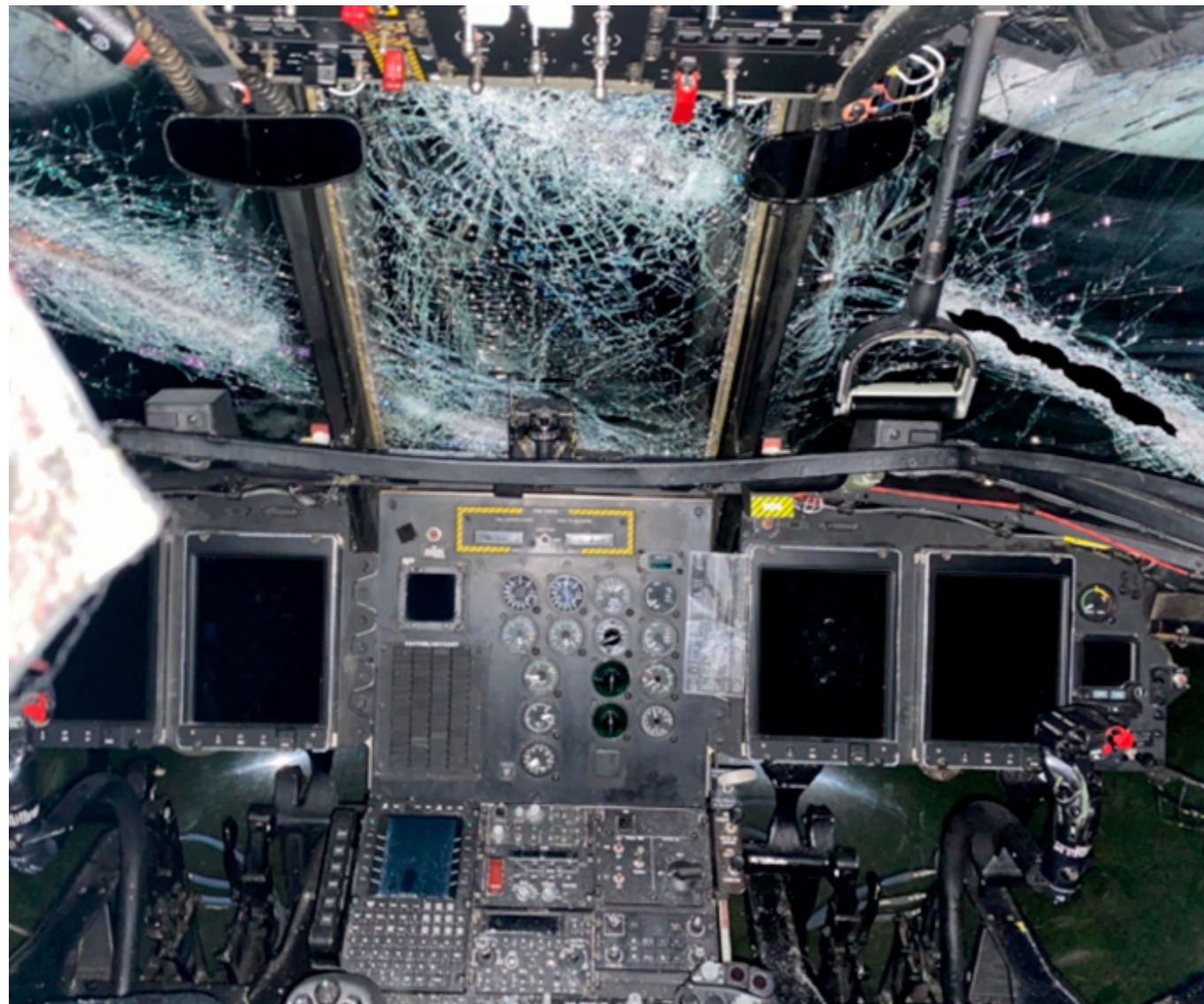
Fig 3. Inside the cockpit showing glass debris and state of windscreens.
