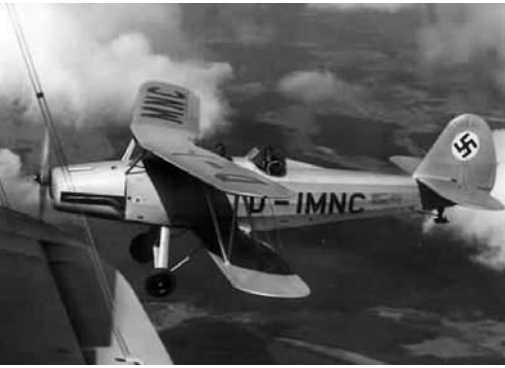
A Gotha Go145 military training aircraft in civilian markings during the mid-1930s
