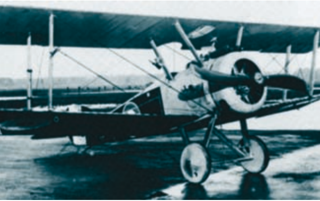
A Sopwith Camel of 1917, carrying the standard armament of two Vickers .303 machine guns (AHB RAF)
