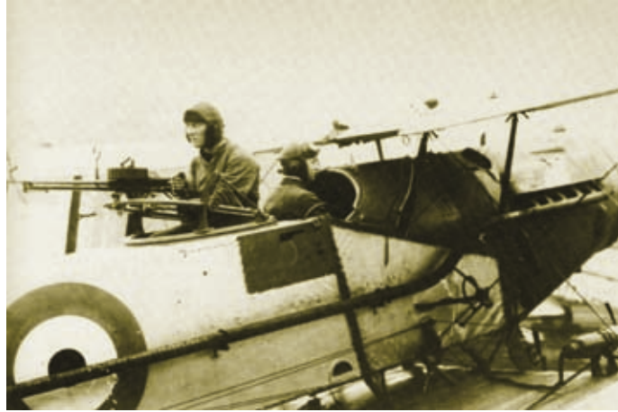
The Bristol Fighter was the most successful two-seat fighter of the First World War. Here a gunner demonstrates the Lewis gun on its ring mounting (AHB RAF)
