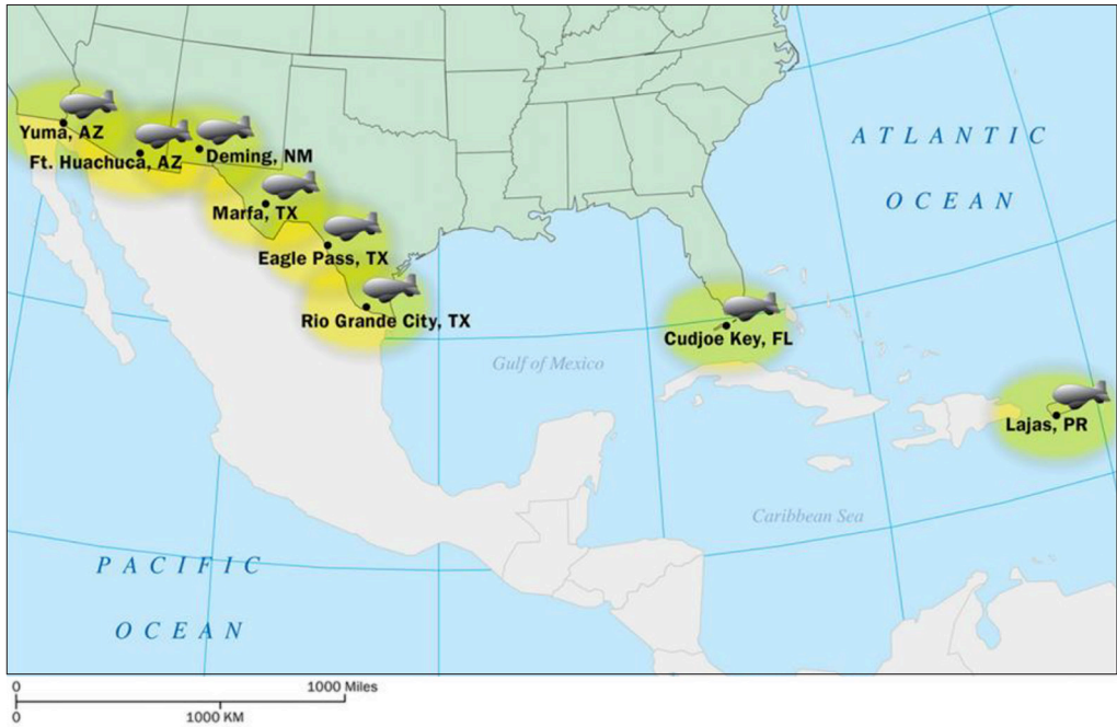
Map 2: Tethered Aerostat Radar Systems coverage in the United States and Caribbean 85
