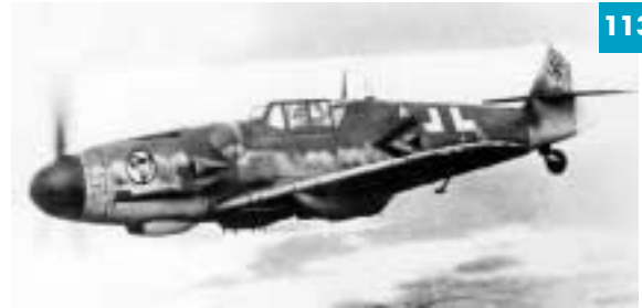
The Messerschmitt 109G formed the bulk of the defending fighter force on 6 March 1944. This example was armed with three 20 mm cannon and two 13 mm machine guns.
