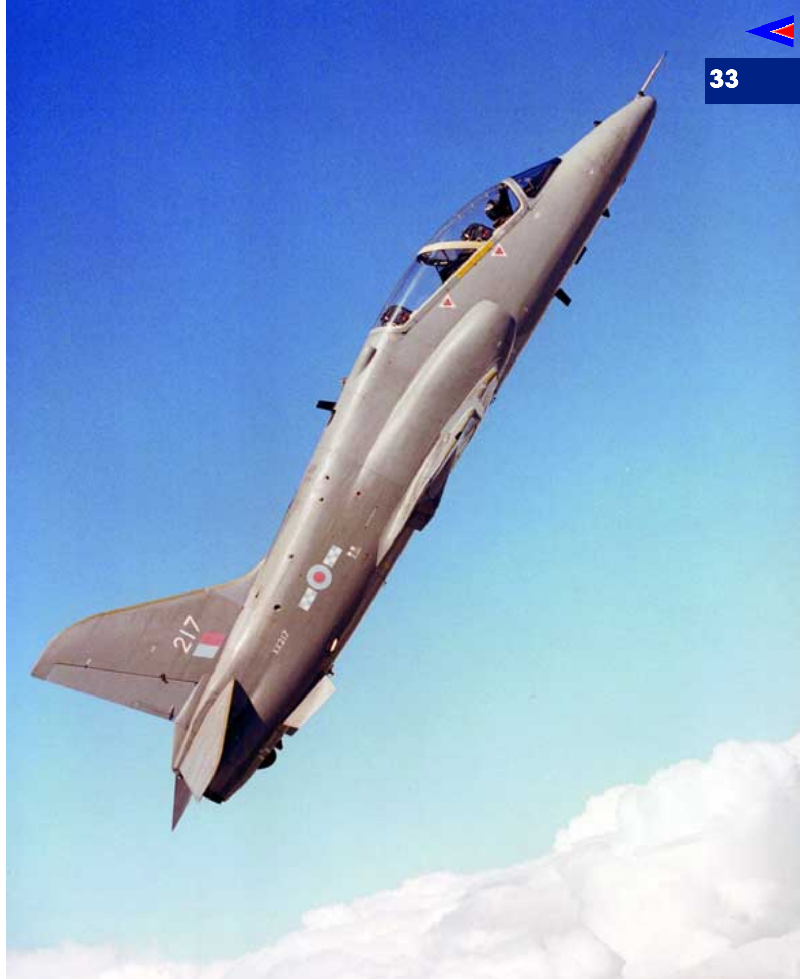
An RAF Hawk T.MK1A. The aircraft can be equipped with wing-tip AIM-9L Sidewinder air-to-air missiles and a cannon pod beneath the fuselage.
