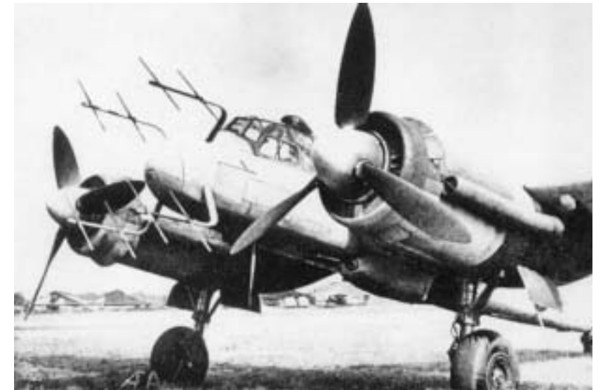
Canted antennas on this FuG 220 reduced interference
