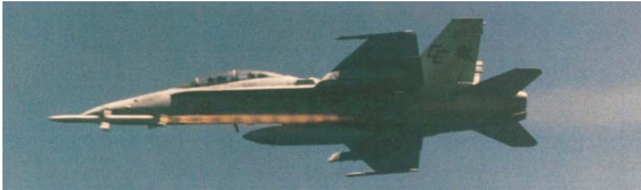
A US Navy Hornet launches an AGM-88 HARM missile. SEAD (Suppression of Enemy Air Defences) enables the missile to reach and destroy an enemy transmitter before it can be shut down
