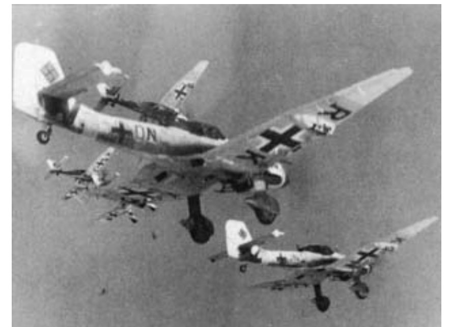
The Luftwaffe disguised some of their aircraft with water-soluble white distemper. Shown are JU 87Ds aircraft
