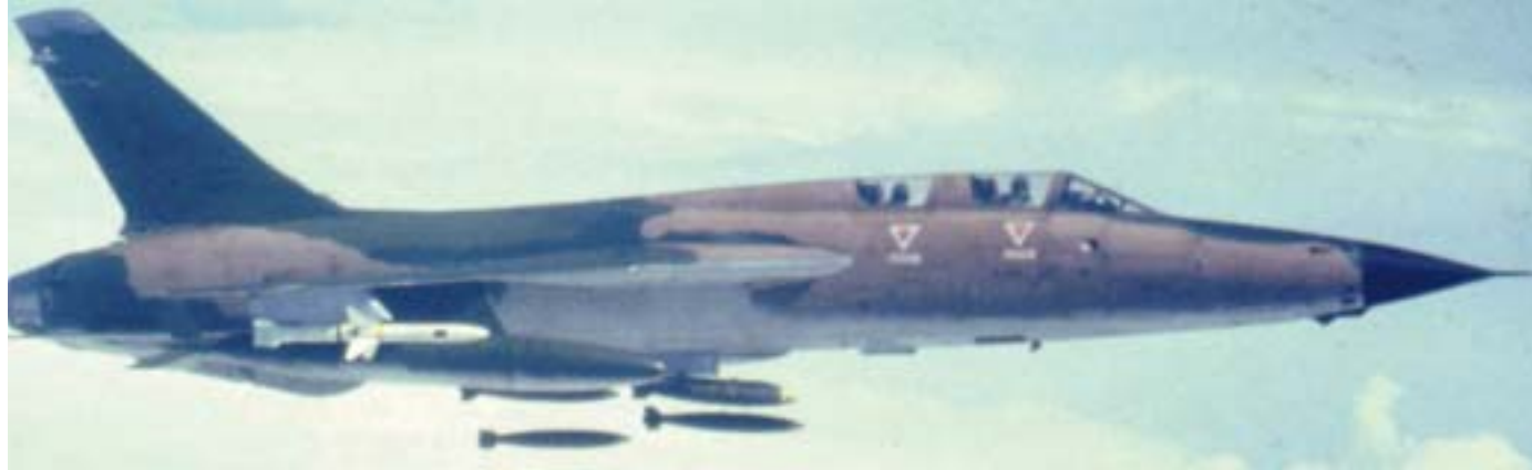
An EF-105F Wild Weasel SEAD aircraft releasing Mk 82 500lb bombs, 1967; note the AGM-45 Shrike ARM on the outboard wing pylon.
