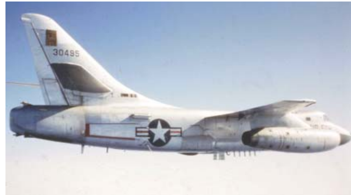
In response to the threat posed by North Vietnamese SAMs and fighters, EB-66 electronic warfare aircraft were used to supplement the jamming pods carried by US strike aircraft during Rolling Thunder.
