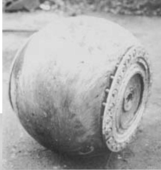
An early version of a Highball used for spinning trials.
