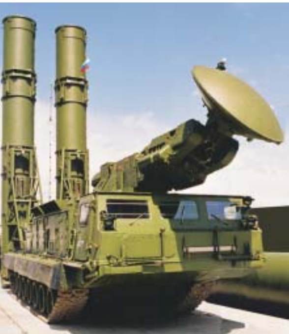
SA-12b 'Giant' SAM launcher with missiles elevated into vertical position and engagement radar at front of vehicle still lowered in travelling position
