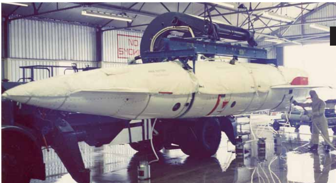
A Blue Steel missile being refueled with high test peroxide (HTP), RAF Scampton
