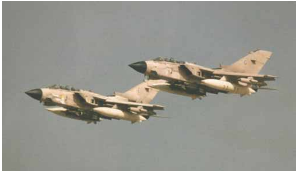
RAF Tornado GR1 aircraft equipped with laser guided bombs
