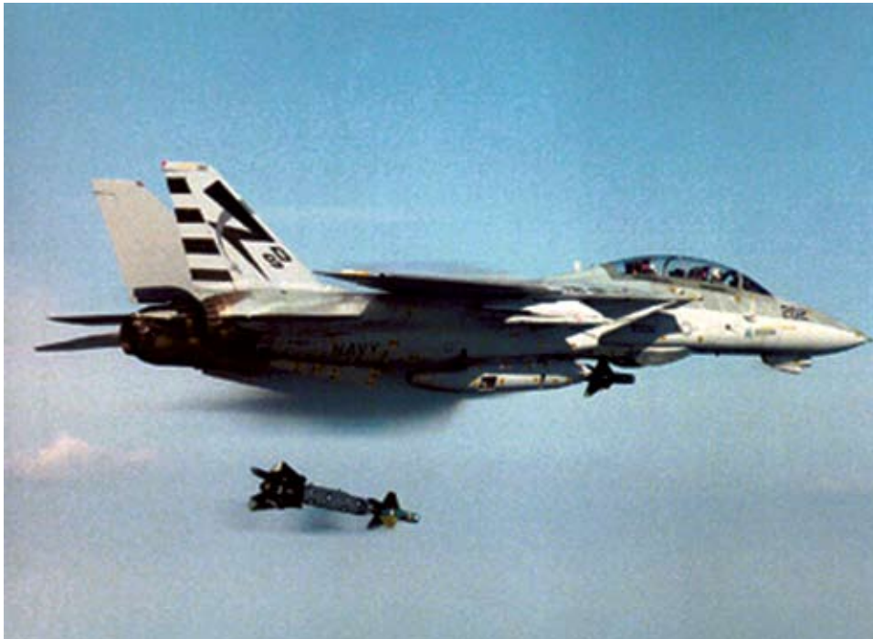
A Grumman F-14 Tomcat of the Naval Air Warfare Center releasing a laser-guided bomb
