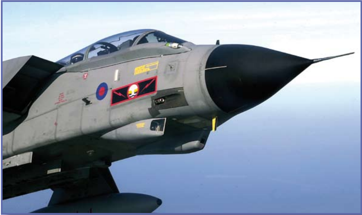
A Tornado GR4 of No 617 Squadron; the muzzle of the 27mm Mauser cannon carried by this aircraft can be seen ahead of the squadron badge (AHB RAF)
