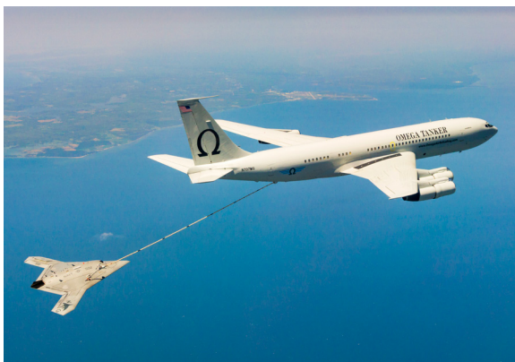
The US Navy’s X-47B UCAS-D achieved autonomous in-flight refuelling on 22 April 2015 – a milestone for aviation, but no indicator that machines are capable of out-reasoning humans. (Credit: U.S. Navy)
