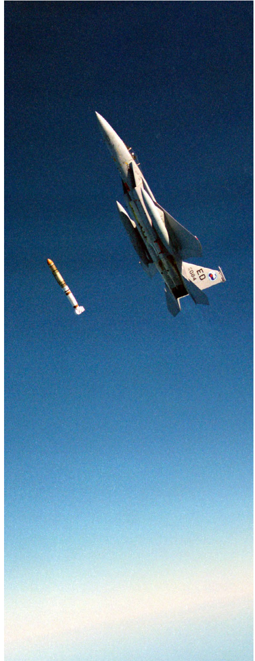
Motor ignition of the ASM-135 ASAT launched from an F-15 Eagle approximately 200 miles west of Vandenberg Air Force Base, CA. (Credit: Paul E. Reynolds, Public Domain, via National Archives Catalog)
