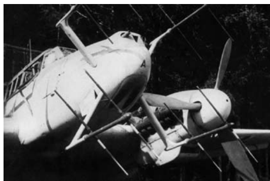
A Bf-110 equipped with SN-2 radar
