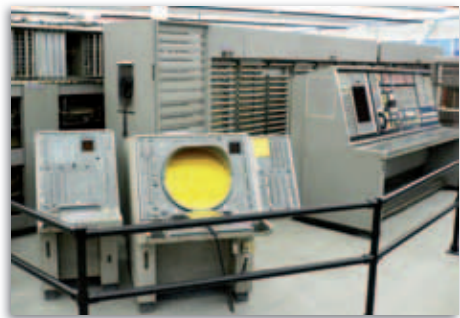
IBMs SAGE is a large semi-automated air defense system from the Cold War era, deployed in 1958, obsolete by 1960.
