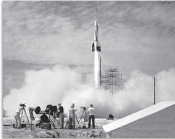
In 1949, the “Bumper-WAC” became the first human-made object to enter space as it climbed to an altitude of 393 kilometers (244 miles). The rocket consisted of a JPL WAC Corporal missile sitting atop a German-made V-2 rocket.
