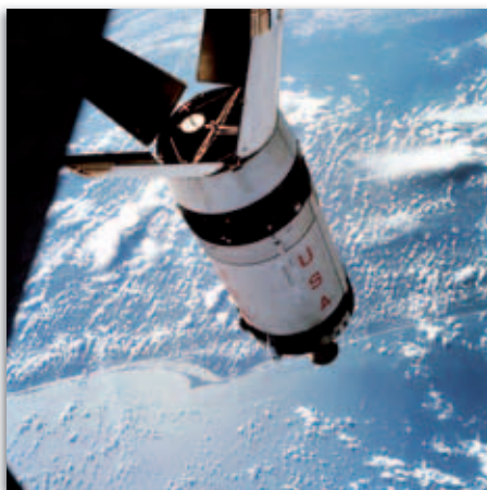
Apollo 7 S-IVB rocket stage in Earth orbit on October 11, 1968. Cape Canaveral and Merritt Island, Florida, can be seen beyond the left side of the lower end of the S-IVB.
