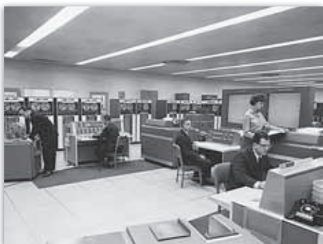
NASA mission control computer room with dual IBM 7090's, apparently taken around the time of the Mercury Atlas 6 (MA-6) mission in 1962.
