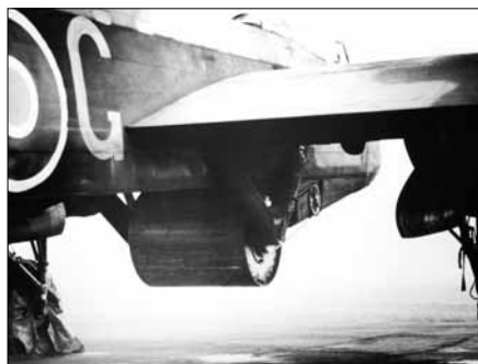
Avro Lancaster with a fixed bouncing bomb under belly
