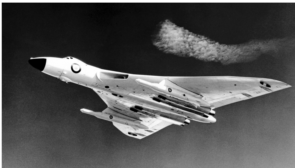
Avro Vulcan B.2, XH537, carrying a pair of dummy Skybolt missiles on underwing pylons. Trials with the missile had started at Avro's Weapons Research Division at Woodford, Cheshire, in November 1961 following an Anglo/American agreement for the supply of up to 100 of the air-launched nuclear missiles which had been proposed as a way of extending the airborne nuclear deterrent into the next decade.
