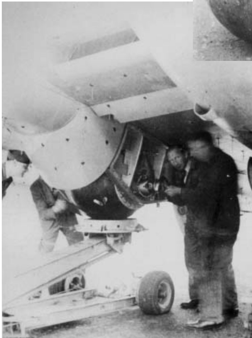
A Highball being loaded into the modified bomb-bay of a Mosquito.
