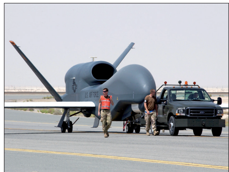
An RQ-4 Global Hawk maintenance team tows an unmanned Global Hawk aircraft
