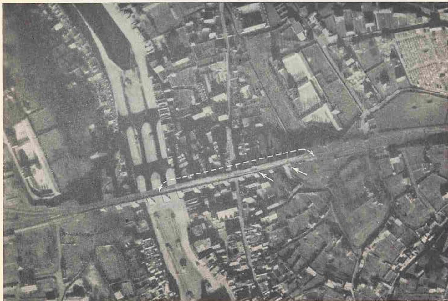
FIG. 18.—Three weeks later both tracks were removed over two-thirds of the length of the viaduct. At least two craters (arrows) can be seen on the viaduct itself and it is believed that the base of one of the piers was damaged. Traffic to Brest had to be diverted by way of the unsatisfactory route through Lorient. (See diagram opposite.)
