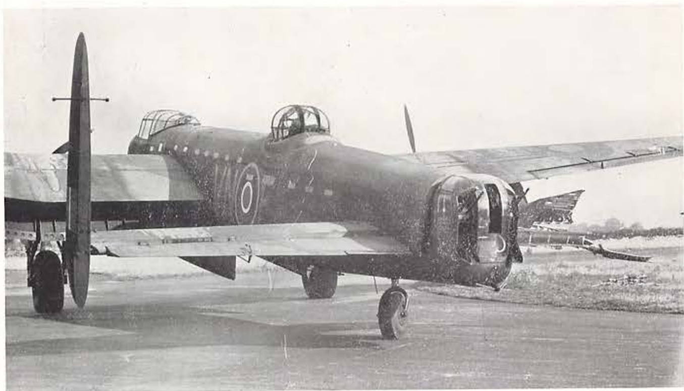
FIG. 13.—This Lancaster of 50 Squadron impacted an unidentified object while over MANNHEIM, on 23/24 September. Although half the tail unit was torn off, the pilot managed to regain control and flew the bomber safely back to base—a distance of some 450 miles. None of the crew were injured.
